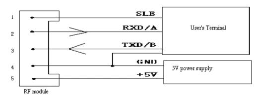
**Remarks:** To avoid to connect the interface reverse and can not communicate, please check and assure the voltage of 3 and 4 pin is existing by using multimeter. If there is one pin that has the voltage, another has not voltage, which means the interface is connected reverse, please change the connection wires between pin 3 and 4.
