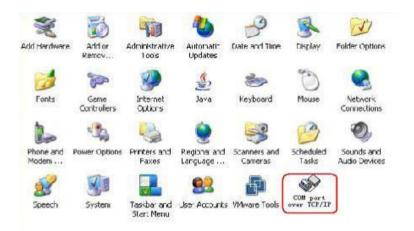
Running the "**COM port over tcp/ip.exe**" application and create virtual COM port communicate with the device on the PC.
