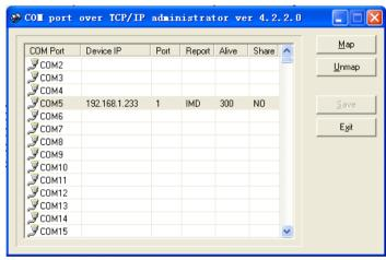
Now, the COM5 can communicate with the terminal on the NO.1 port of the device.
