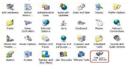
Running the "COM port over tcp/ip.exe" application and create virtual COM port communicate with the device on the PC.
