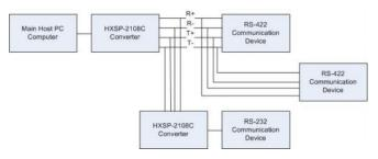
(2) When the HXSP-2108C connects as RS-232/RS-4485, the device connects as RS-485 connection method.
