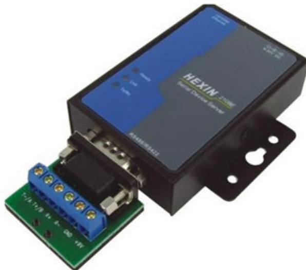
HXSP-2108E-B RS-485/RS-422 to Ethernet TCP/IP Serial Device Server
